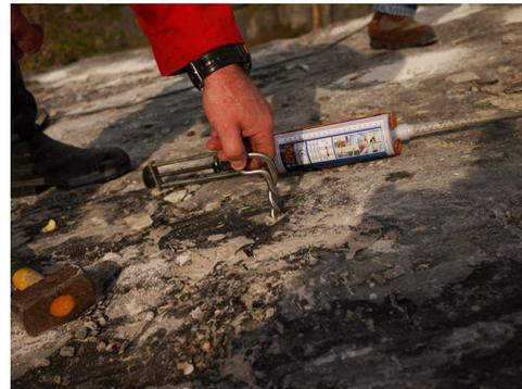
During the test period it became apparent that the chemical anchor mortar had not thoroughly mixed during application into a hole. The peak load to remove this anchor was 36KN. RAWL have been contacted and from the information supplied by us have initiated an investigation.
