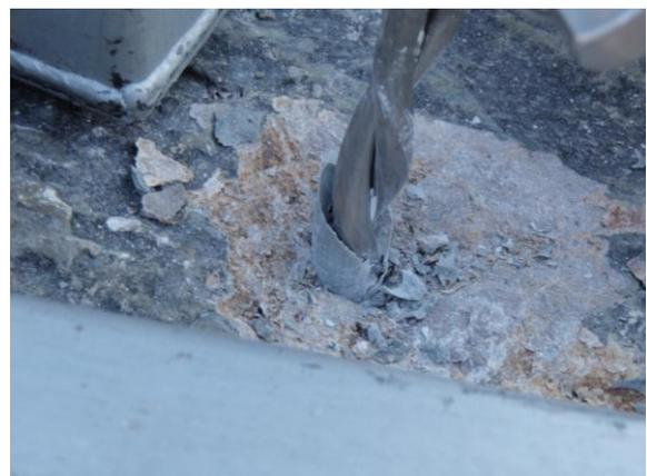
An interesting observation was that the anchors were still holding only a little less than the peak load when half to two thirds of the anchor had been extracted. Whilst no meaningful conclusions can be drawn from the extraction of six bolts it would appear that, because of the styrene, mean failure loads are 10kN higher with the KMR resin.
