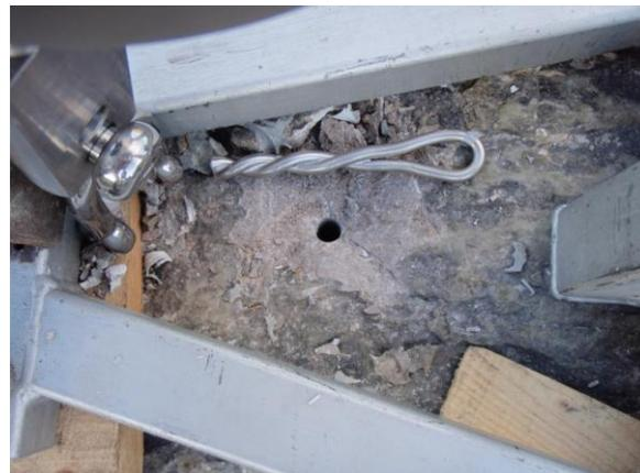
The distortion loads were virtually identical on both resins. However, the mode of failure has changed. Normally the mode of failure is the anchor to resin bond. In most cases the substrate failed and the resin/rock bond with it. During one of the tests the mode of failure was rock cone fracture subsequently followed by the failure of the resin to rock bond.
