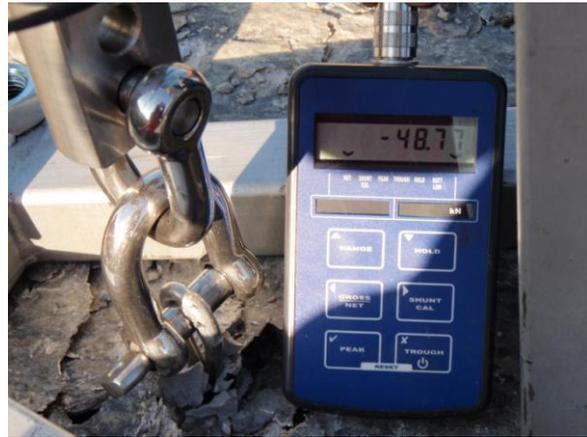
Another interesting observation was that the shank of the Bolt Products anchor unwound and elongated under loads approaching 50kN. (5<sup>th</sup> anchor from right picture below).
