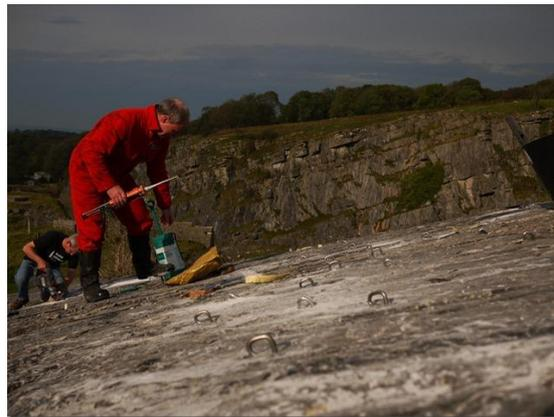
During the test period it became apparent that the chemical anchor mortar had not thoroughly mixed during application into the hole. This resulted in two relatively low readings. Anchor test number 10 was extracted using 26KN. And anchor number 13 was extracted using 18KN. On closer inspection of the chemical anchor mortar it was granular which could indicate that thorough mixing had not occurred, or it require a longer curing time.
