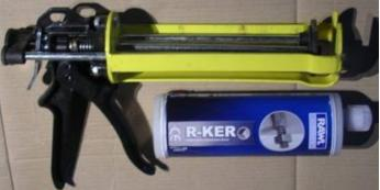
FIS V uses a side-by-side cartridge made up of one cylinder holding the polymer blend and another smaller cylinder attached to the side which holds the hardener. R-KER uses a coaxial cartridge where the smaller cylinder is within the larger cylinder. The two systems require different guns.
