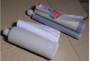
There is a piston in each of the cylinders. The coaxial cartridge has a piston like a doughnut. The side-by-side cartridge gives a 5:1 mixing ratio and the coaxial cartridge gives 10:1. It is possible to peal back the labels and see the components through the translucent plastic.
