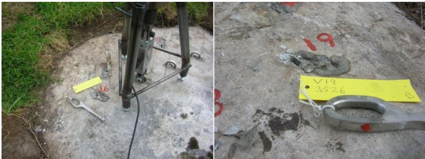
Each tested anchor had a label attached recording its number, the peak load and the resin cartridge.
