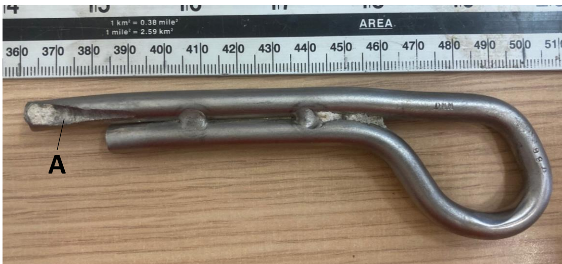
Figure 2 DMM 98A Left side view. Note drill marking at the end of the leg 395-360mm
