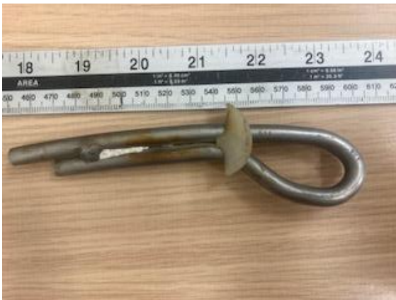
Figure 10 DMM Anchor with distorted head due to extraction, without drilling.
