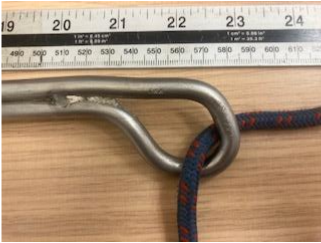
Figure 9 DMM 98A with 6mm cord layed into the grooves in the inner curvature of the anchor.
