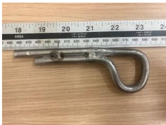
Figure 11 DMM anchor without much distortion of head but lots of drill damage.
