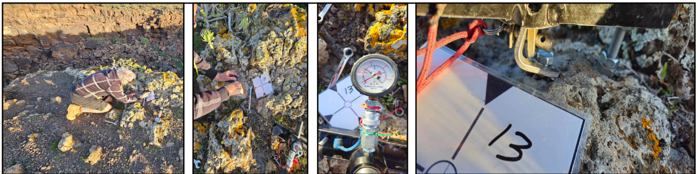
Fig. 8a – 8c showing the location of test 13, welded AA lava Fig. 8d showing failure at 5Kn at second time re-use of the hole by a MMS anchor
