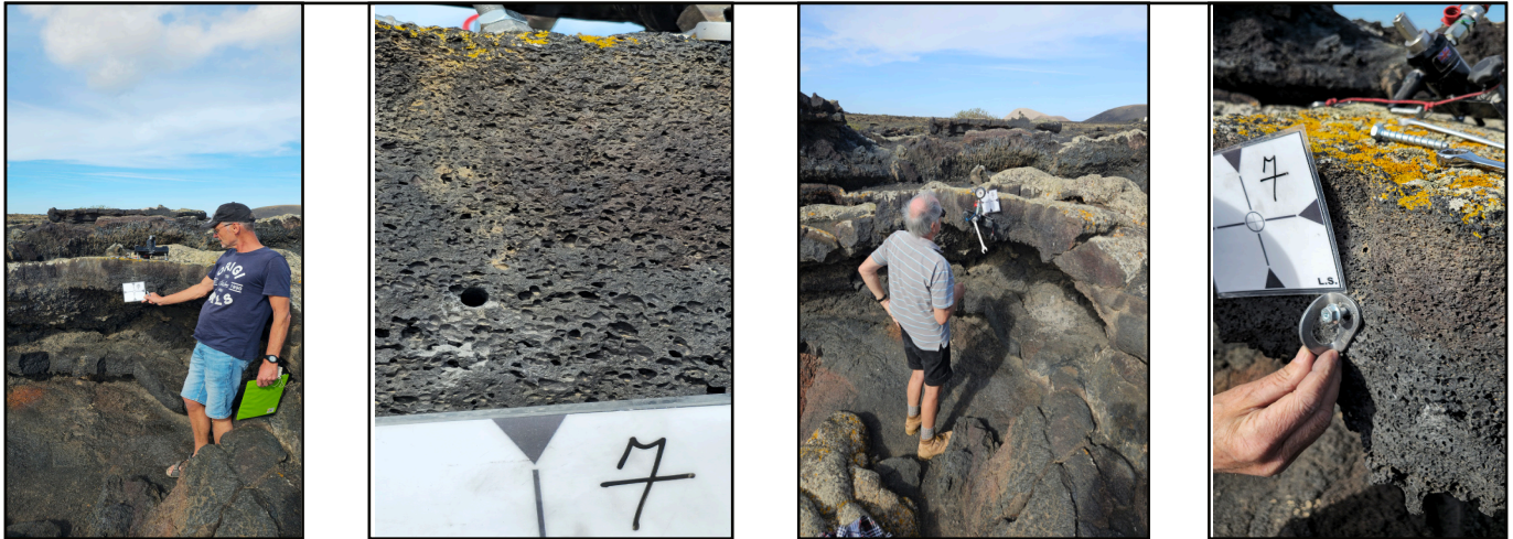
Fig. 7a, 7b and 7c showing location of test site 7: At the side of a Homogeneous looking pahoehoe lava slab . Fig. 7d showing failure at 5Kn. at second time re-use of the same anchor.
