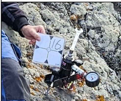
Fig. 9a – 9c showing the location of test 16, clasted basalt (welded small rocks). Failure at 4Kn.
