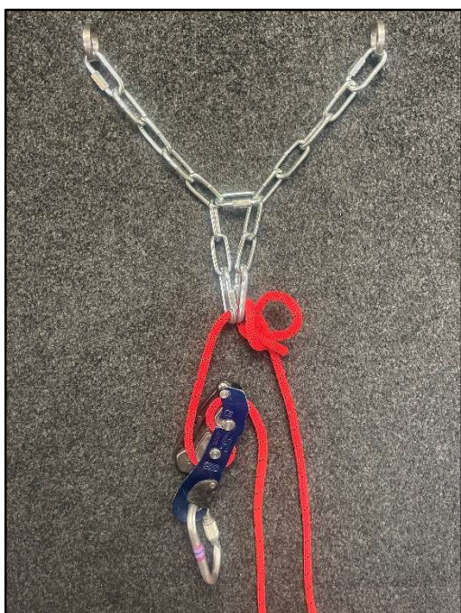
Chain rigging for pull down
