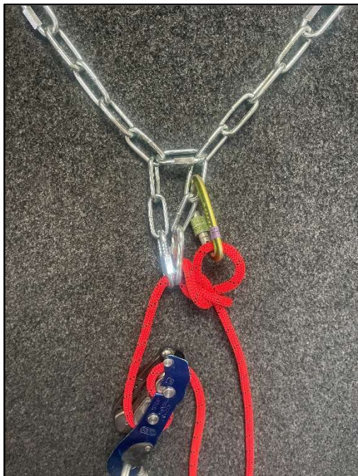
Chain rigging 'locked off'
