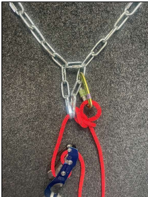
Chain rigging 'locked off'
