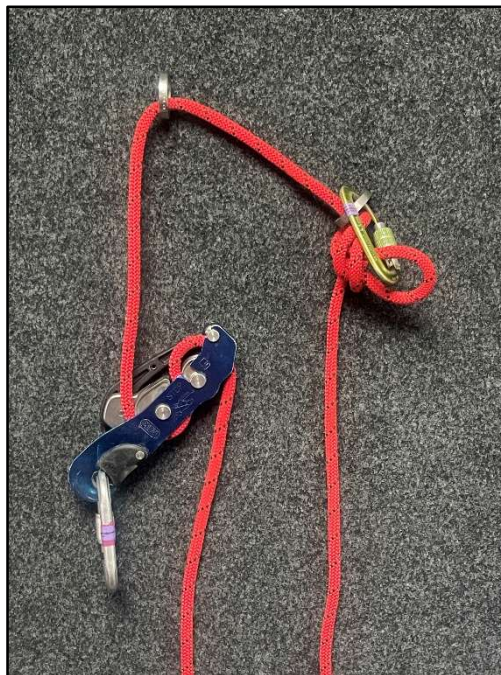
Anchor rigging 'locked off'
