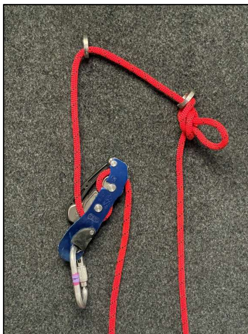
Anchor rigging for pull down
