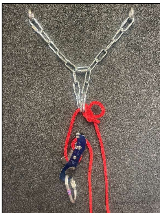
Chain rigging for pull down
