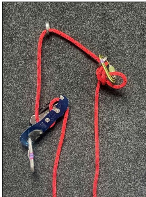
Anchor rigging 'locked off'
