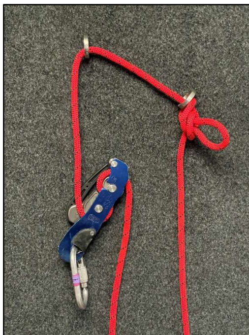
Anchor rigging for pull down
