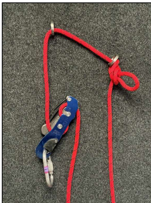
Anchor rigging for pull down
