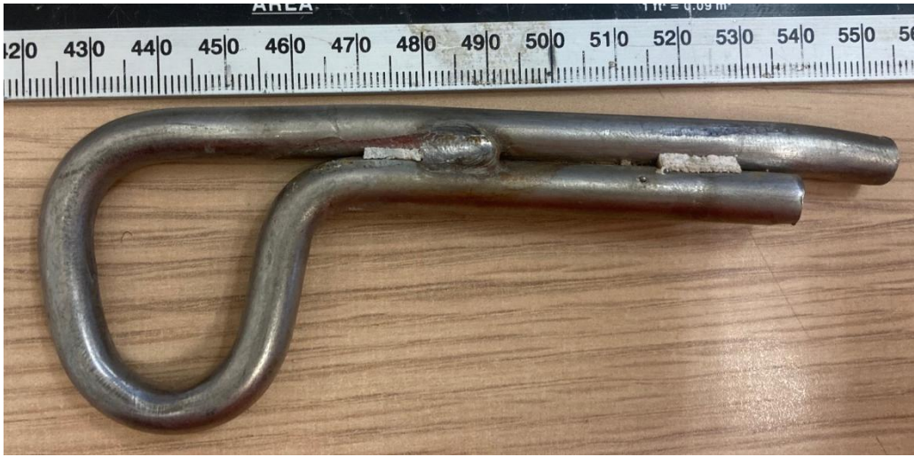
Figure 6 Anchor Z Right side view note drill marking down leg of anchor, 480-490mm at weld.
