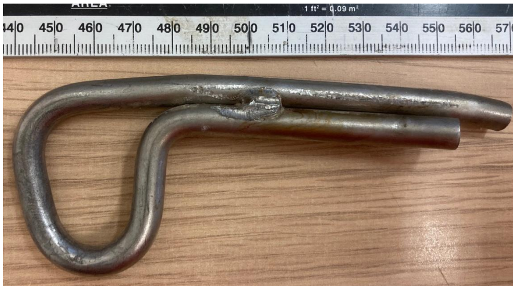
Figure 4 Anchor Y Right side view note drill marking down leg of anchor, 490-510mm.
