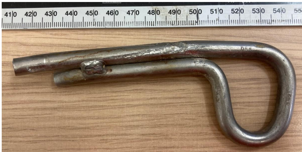
Figure 1 Anchor W Left side view note drill marking down leg of anchor, 420-425mm and 450-500mm.
