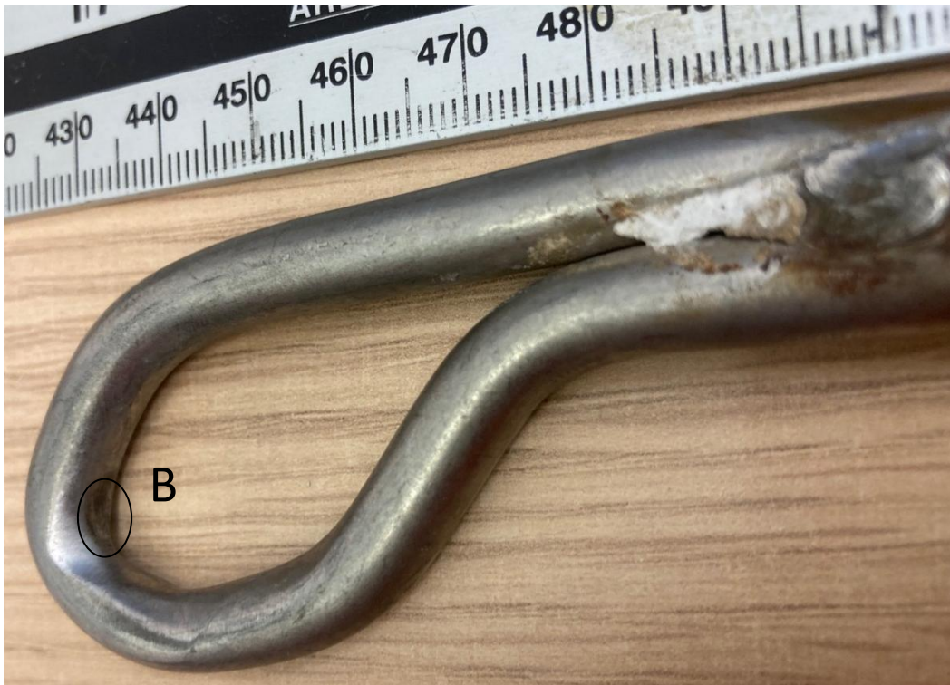
Figure 12 Anchor X Right side view, note small flattening of ridge in the inside curvature by the puller, deep grooves are worn into the anchor.
