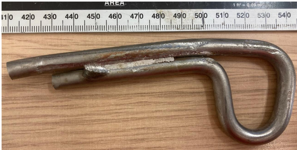
Figure 3 Anchor Y Left side view note drill marking down leg of anchor, 420-500mm and 530-535mm.
