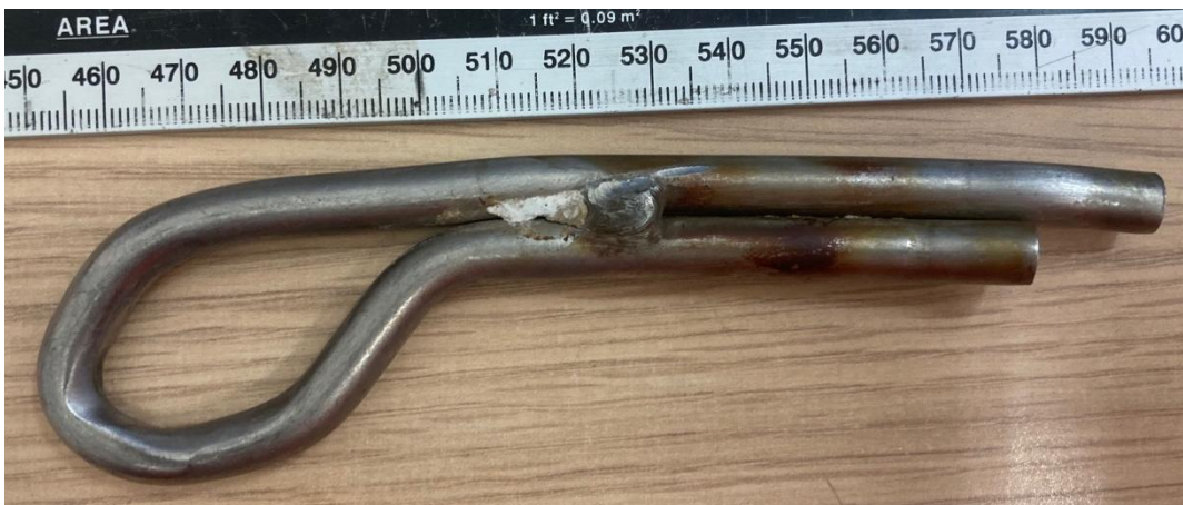
Figure 8 Anchor X Right side view note drill marking down leg of anchor, 510-535mm.
