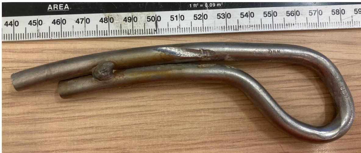
Figure 9 Anchor XX Left side view note drill marking down leg of anchor, 495-520mm.
