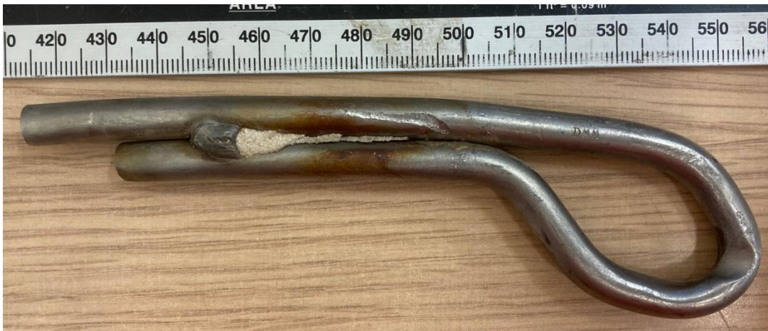
Figure 7 Anchor X Left side view note drill marking down leg of anchor, 475-495mm. Note also the brown staining on the legs for the anchor.
