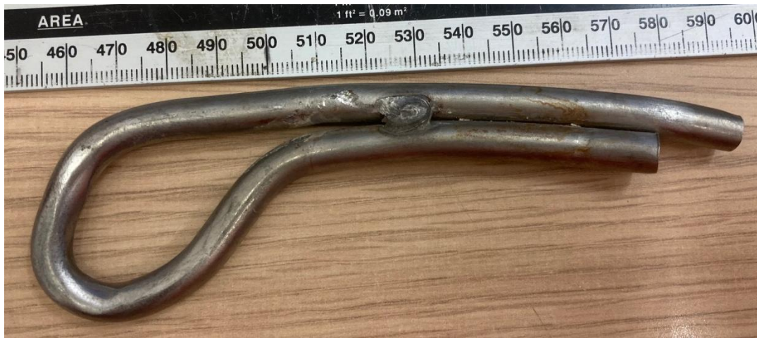
Figure 10 Anchor XX Right side view note drill marking down leg of anchor, 510-520mm.
