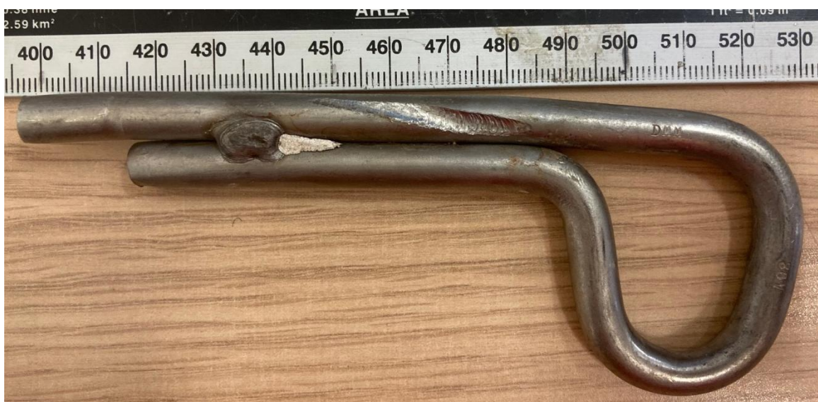
Figure 5 Anchor Z Left side view note drill marking down leg of anchor, 445-485mm.
